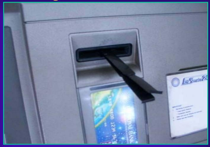
The trap is then inserted into the ATM slot. Care is taken not to insert the entire film into the slot, the ends are folded and contain glue strips for better adhesion to the inner and outer surface of the slots.
