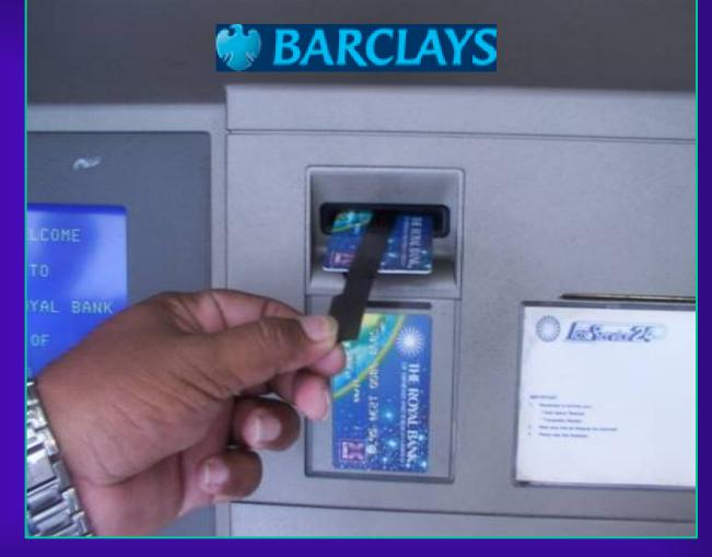
As soon as the "Customer" has gone, and they have your PIN, The thief can remove the glued trap, by grasping the folded tips, he simply pulls the trap out that has retained your card..
